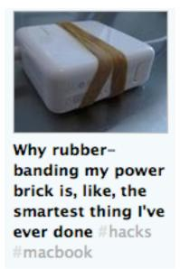
As beautifully designed as the MacBook power cord assembly is, it has two fundamental design flaws. One is that the plug-side cord is HEAVY. Combine this with the brick's slippery shiny surface, and you have a recipe for a plastic block being dragged off a table by a cable that's slung like a catenary between the outlet and the table's edge. [If] you [rubber band it] ... the brick doesn't move at all.
